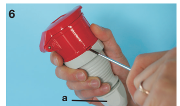
To disassemble first unscrew the cable gland (a). Then press the screwdriver (blade width 3.0 mm) deeply into the opening slot of the back part. Turn screwdriver clockwise to unlock the parts again.
