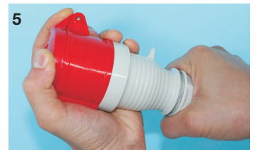
Finally tighten the cable gland (torque at least 4 Nm) - ready.
